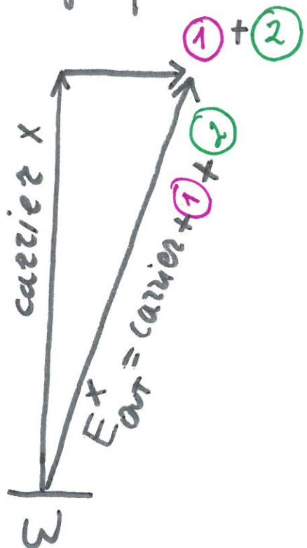
Let's see what happens to  $E_{\text{out}}^y$ . The carrier has a phase  $\beta = \omega \frac{2Ly}{c}$  but the phase related to the GW has to be the same  $\gamma$ :
